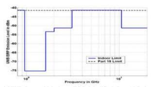
Fig. 1 UWB Spectral Mask per FCC (Modified) Part 15 Rules [1]
