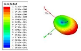
Fig. 6 Gain of micro strip patch antenna is 1.4162 dB
