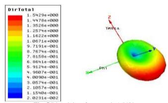
**Fig. 5** Directivity of antenna is 1.5429
