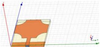
Fig. 2 Geometry of rectangular patch corner cut antenna
