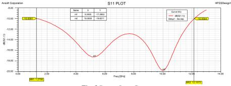
Fig. 3 Return Loss Curve
