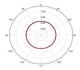
Fig. 9 Radiation Efficiency at different 'Phi' (10GHz)
