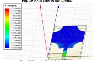
Fig. 12 Electric field of the antenna
