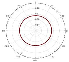
Fig. 8 Radiated power at different 'Phi' (10GHz)
